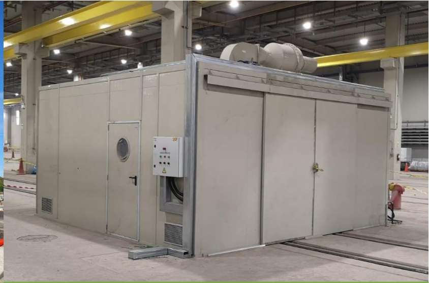
Bogies washing Cabin at Lima (Peru)
