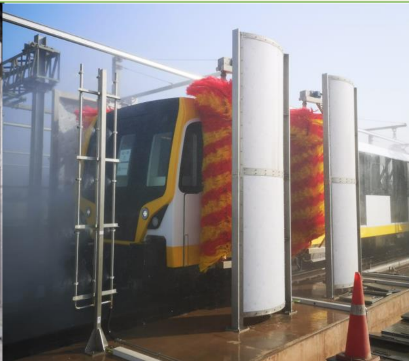
Train Wash Plant at Lima (Peru)
